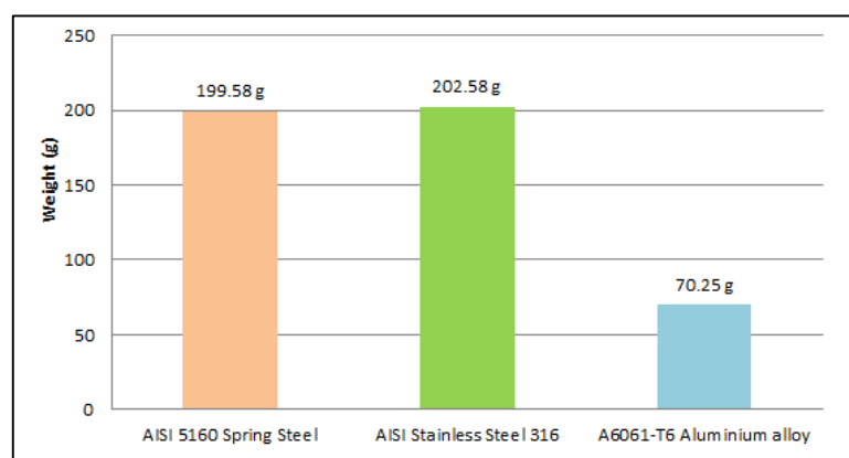
Figure 11. A graphical comparison of sickle weight with different metals.
