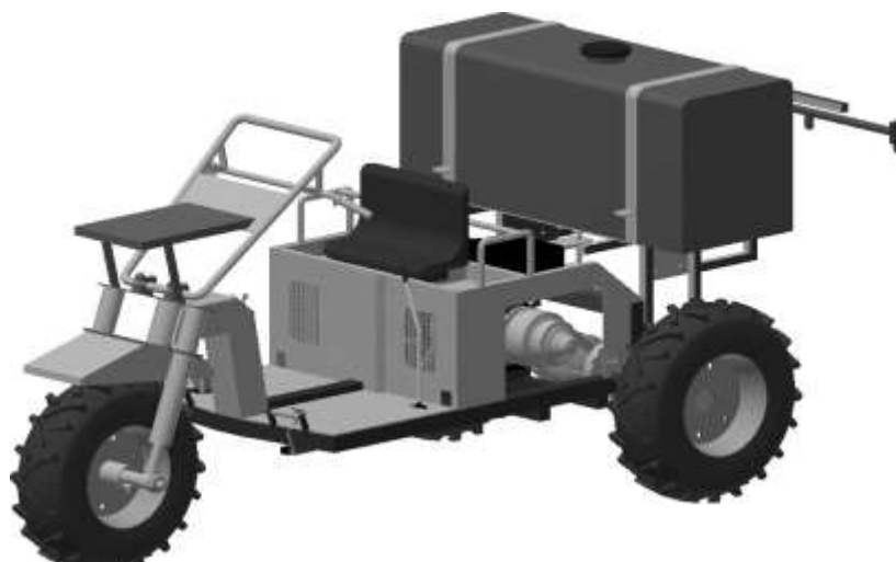
Figure 1. Three-wheel type machine with a solar charging and electric spraying system.
