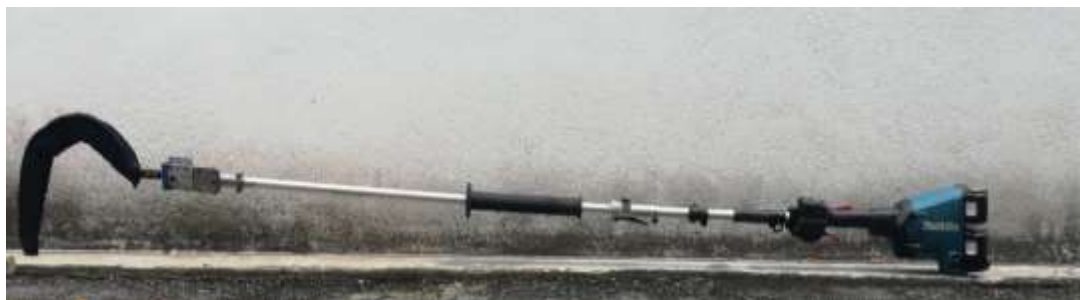
Figure 1. A motorized oil palm cutter or CANTAS which was developed by MPOB.
