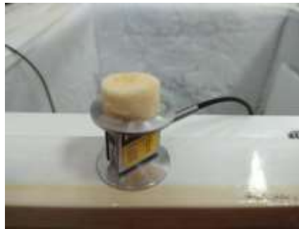
Figure 2. Frozen confection sample with a diameter of 1.5 cm and height of 0.75 cm.
