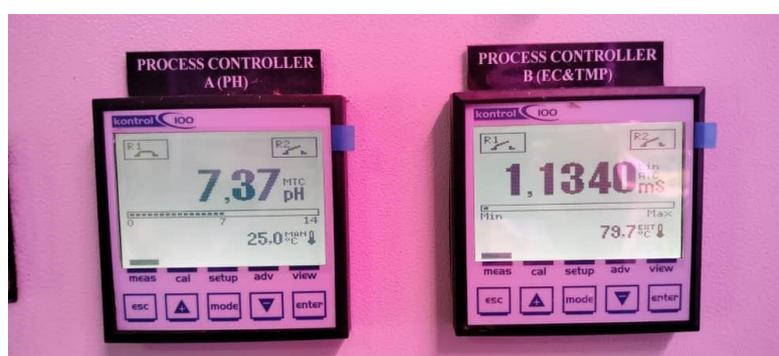
**Figure 4.** EC, temperature, and pH sensor system.
