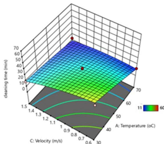
**Figure 4.** Response surface plot illustrating the cleaning time of milk fouling deposit influenced by the combined effects of fluid velocity and temperature.
