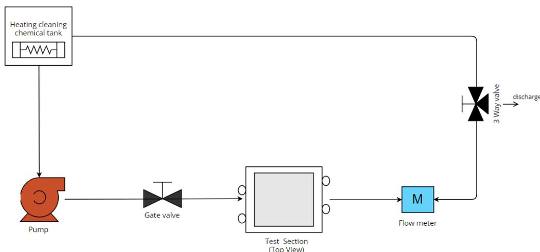
**Figure 2.** Process flow diagram of the cleanability experiments.
