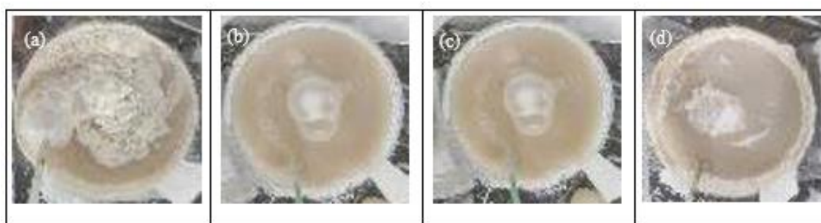
Figure 7. Foaming of diluted FPW aerobic digestion added with biosurfactants after aeration for (a) 30 mins, 0.04 g RL/g TSS; (b) 2 h, 0.04 g RL/ g TSS; (c) 30 mins, 0.15 g SP/g DS; (d) 19 h, 0.15 g SP/g DS.
