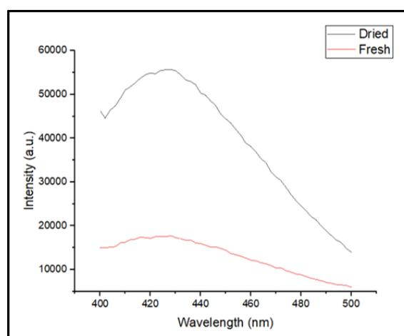
**Figure 5.** Emission scan of PL intensity of PM-AgNPs
